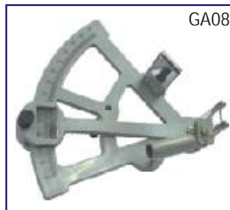
GA08 SEXTANT MODEL : with frame, divided arc fitted with vernier, reading to 1-10 degree sighting hole, glass mirror. Rs. 649.00
