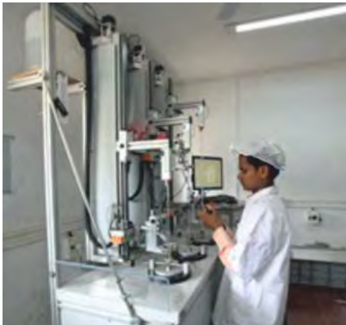
Computer controlled automatic calibration machine with optical laser beams to prevent human error and ensure highest level of accuracy and precision
